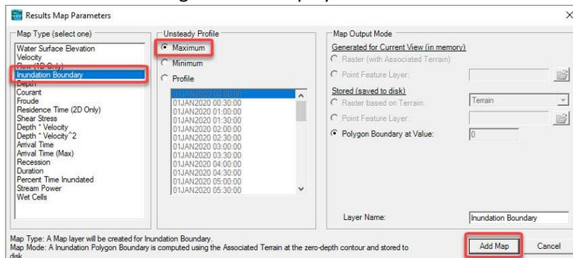
3. You can create a new layer displaying any of the Map Type information, at any particular time. To generate the maximum inundation
