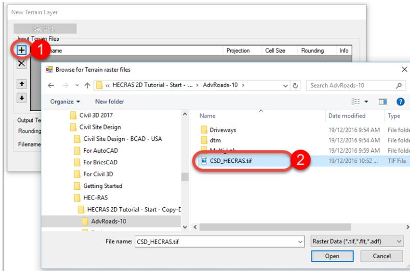
12. Click on + to add a new data source for the terrain. Navigate to the output location of the .tif and open that file
