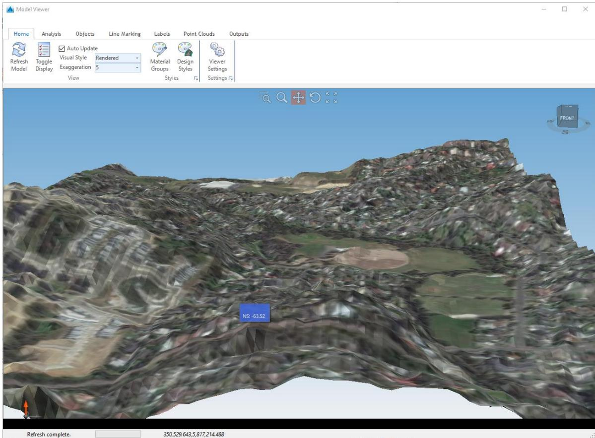
*Note: in the above image the exaggeration has been set to 5 to accentuate the shape of the terrain. Exaggeration must be set to 1 before exporting*
