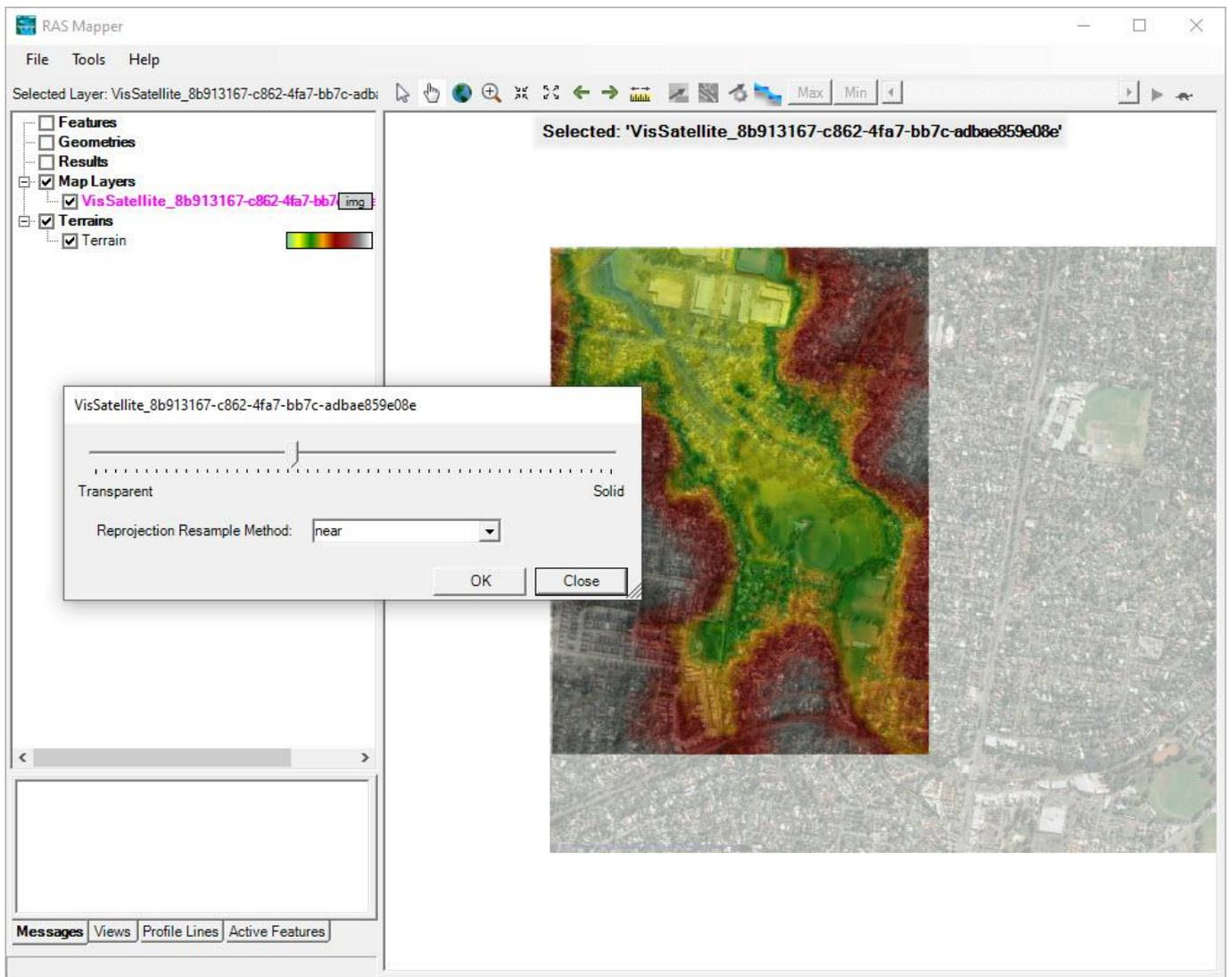
After importing data into RAS Mapper, it will become available in the HECRAS Geometry Editor. In here you can assign flood data along the boundaries, establish the model grid size for flood analysis, edit the surface breaklines, assign different surface Manning's n values and more.
