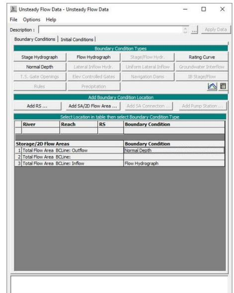
31. Under Add Boundary Condition Location, click on **Add SA/2D Flow Area...** to include the Total Flow area
