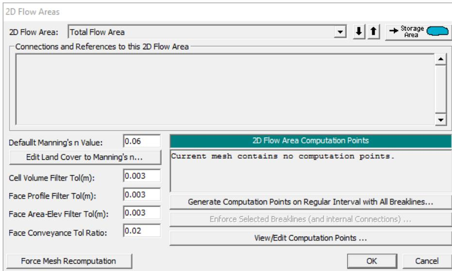
21. Click on Generate Computation Points on Regular Interval with All Breaklines...
