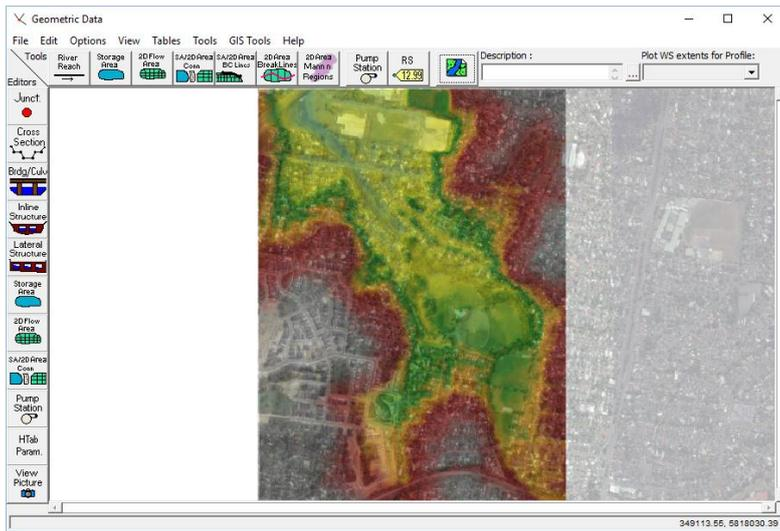
The linework in your original drawing can be included in the Geometric data as a layer, after exporting it out from the drawing in an appropriate format for HECRAS.
