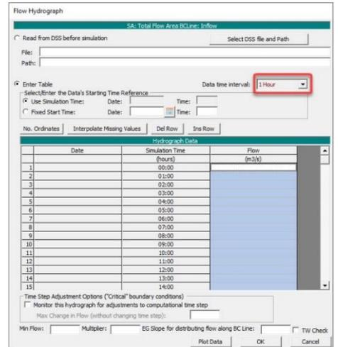
For this purpose, you may wish to open the file Storm Input Calculator.xls file located in the same directory as the source drawing. In this file, you can type in the Minimum and Maximum flow values at the top of the form and it will populate values for 1hr increments.
