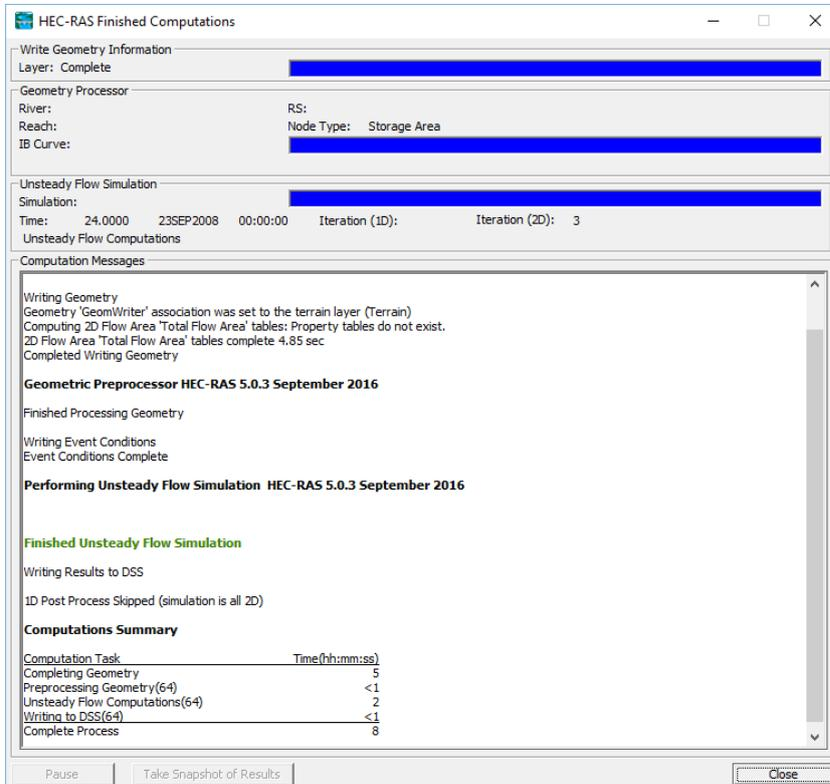
If you receive any information in **red** text, it is likely that some data has not been saved, data hasn't been fully added or there is an error in the mesh or data input.
