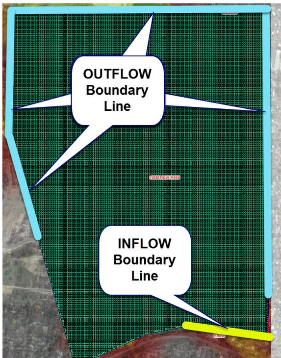
Note that in the geometry editor you can incorporate both 1D and 2D flow zones into a single model for analysis. Additionally, boundary conditions can be set within the 2D area to represent different hydraulic behaviours. After setting up the surface and boundary conditions, you can move onto assigning the flow conditions.
