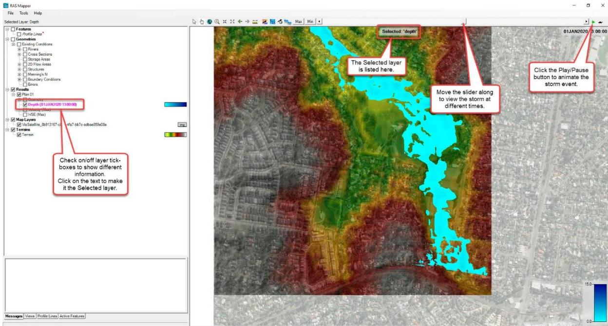
Tick on the Depth layer to show the depth of water. Click on the Depth (Max) text to make it the Selected layer and use the slider at the top to change the flow time to see development of flow over time. The play button will animate the flow.
